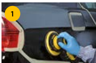
1 Preparation of adjacent panels and panel blend. Use Abralon® grit 1000 disc damp or Polarstar®/Microstar® disc with interface pad dry.
