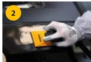
2 Shape and level body filler. Use net strip P80 or P120 with sanding block or Mirka® OS 383 machine for smaller areas.
