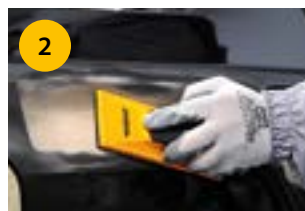
2 Fine sanding of body filler and feather out. Use net strip P180-P240 with sanding block or Mirka® OS 383 machine. >>> Check repair area, if required fill pinholes with a fine polyester filler.
