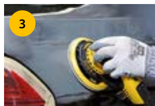
3 Machine sand the area. Use net disc grit P500 + interface pad or Gold Soft Grip disc P500.
