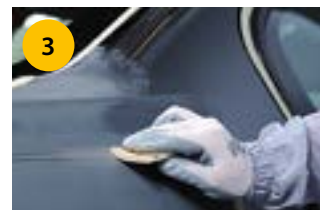
3 Sand edges and hard to reach areas with Goldflex-Soft P500.
